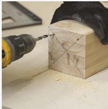
2 Reaming holes for wood screws.
