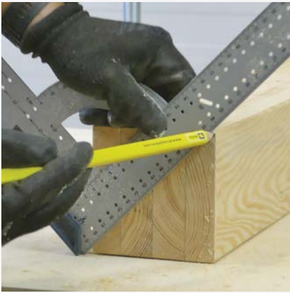
1 Determination of post diagonals.
